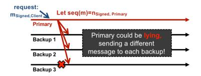
Phase 2: **Prepare:** replicas exchange/disseminate request they got from the primary to each other. They need to exchange these messages because the leader cannot be trusted, so he could have sent n, m to one set of replicas and n, m' to another set of replicas. Replicas wait to receive 2f+1 confirmations for the same <n, m>. If they get this, they are "ready to commit."
