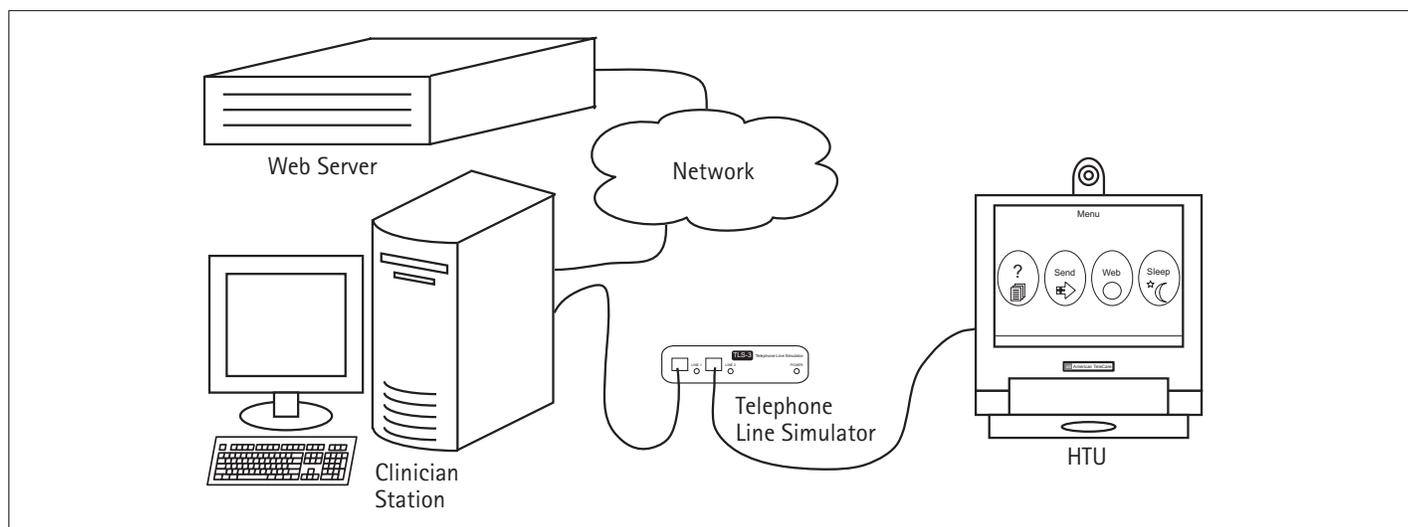
**Fig. 3.** Experimental testbed showing trainer's workstation, Web server, telephone line simulator, connected to home telemedicine unit (HTU).
