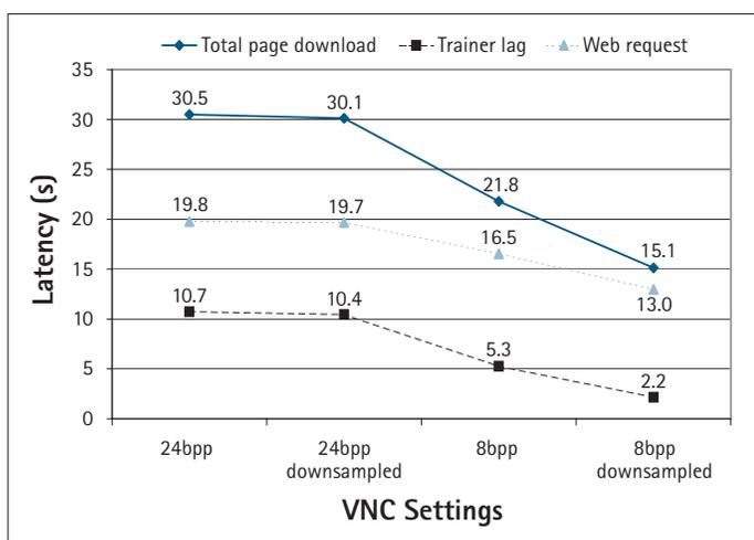
**Fig. 4.** Measurements taken from packet captures, varying the bit depths and downsampling factors.
