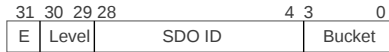
Figure 4: CleanOS Taint Tag Structure. We impose a structure on TaintDroid taints to support arbitrary numbers of taints.
